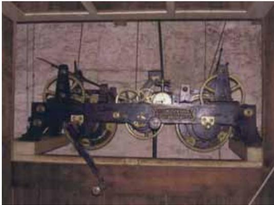
The clock mechanism with the original turning handle on the left hand side © St Mary's PCC 2008
